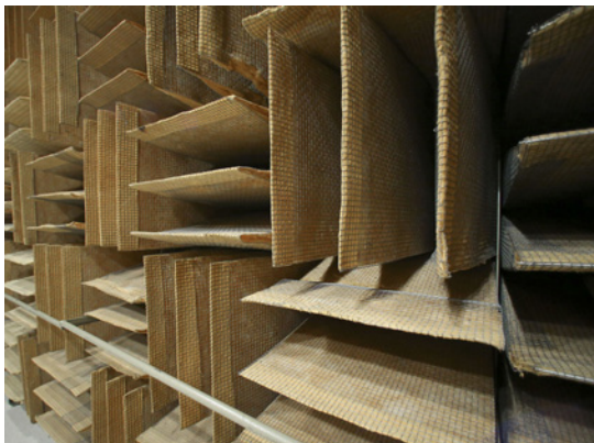
The insulation baffles are shown inside the anechoic room in the acoustics lab at Trane Co. The room is designed to completely absorb reflections of sound.
